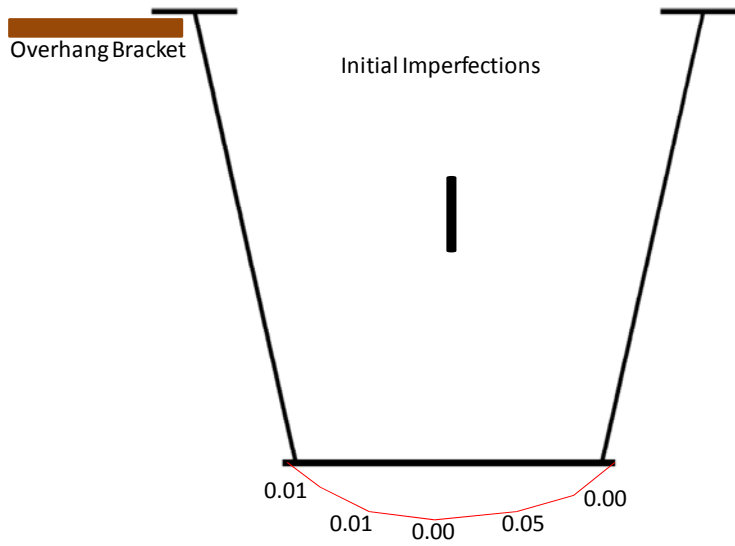
Figure 5-9 Int. Girder Bottom Flange Initial Imperfections
