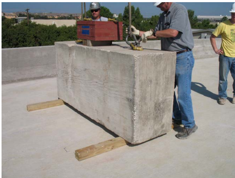
Figure 4-18 Live Load Simulation - Front Axle
