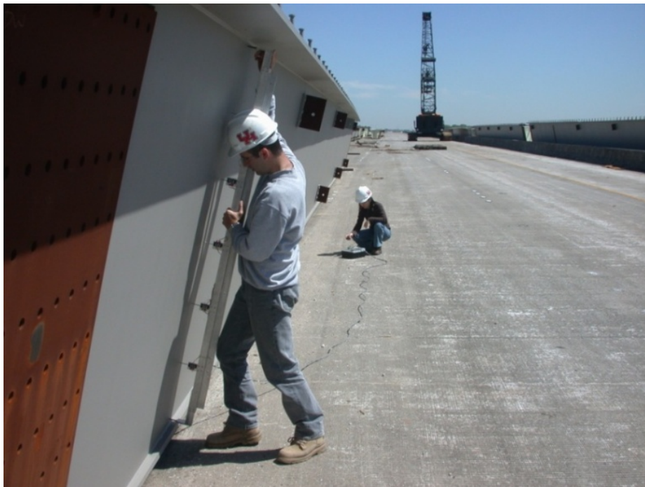
Figure 3-21 Measuring Web Imperfections (Mercan, 2005)
