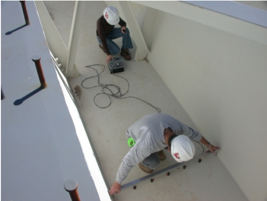
Figure 3-22 Measuring Bottom Flange Imperfections (Mercan, 2005)
