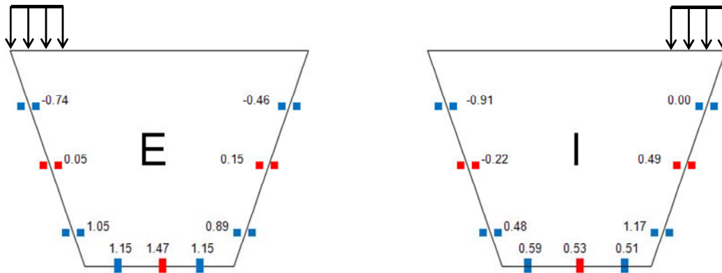
Figure 4-15 Average Stress Changes due to East Rail (ksi) Section A
